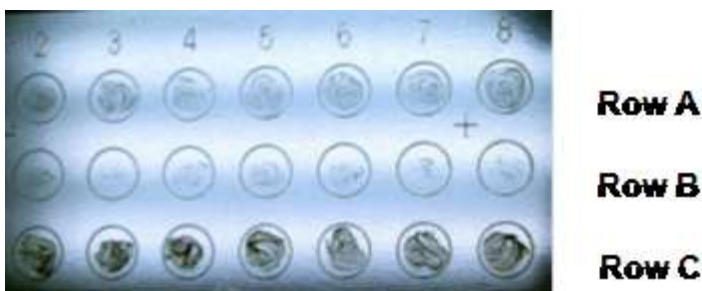
Figure C-1 Ideal (row A) and suboptimal (rows B and C) amounts of biological material on a MALDI target plate
